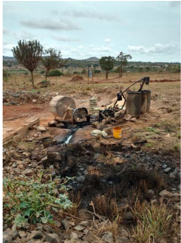
Diesel spills from a generator on a mineral processing site (Mara, 2017 – Photo: IPIS)
