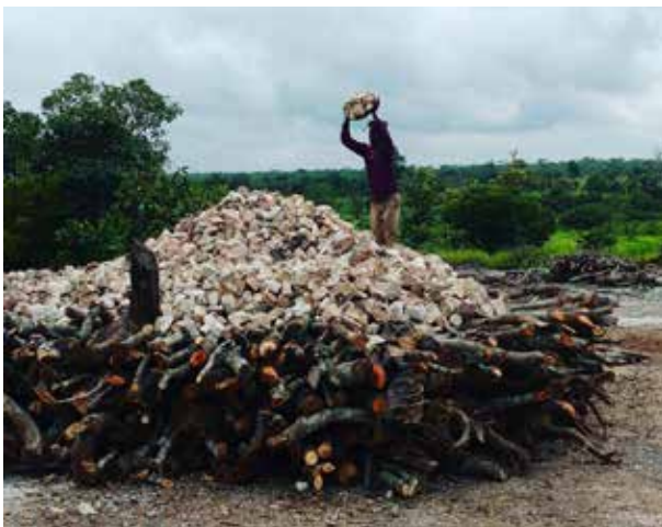
Workers crushing limestone into aggregates (1), Truck picking up aggregates for construction (2), Worker adding limestone on top of a woodpile (3), A pile of coarse slaked lime (4) (Kigoma, 2018 – Photo: IPIS)
