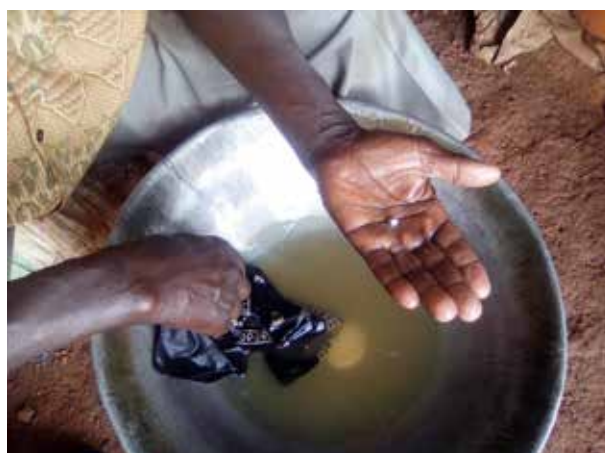
Processor amalgamating gold with mercury (Mara, 2018 – Photo: IPIS)
