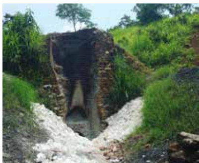
Brick limestone kiln (5), Lime milling (6), Lime packaging in branded bags (7) (Kigoma, 2018 – Photo: IPIS)
