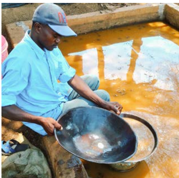
Processor using mercury to extract gold from its ore (Shinyanga/Geita, 2018 – Photo: IPIS)
