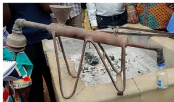
Retort used to capture and recycle mercury fumes during the burning of the amalgamate (Geita, 2019 – Photo: IPIS)
