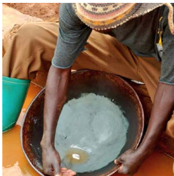
Processor using mercury to extract gold from its ore (Shinyanga/Geita, 2018 – Photo: IPIS)
