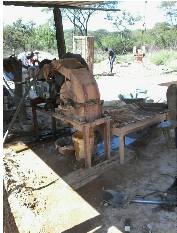
Picture 6: Example of processing done in a gold mining site that treat 60 tons of ore per month and using both mercury and cyanide. 11
