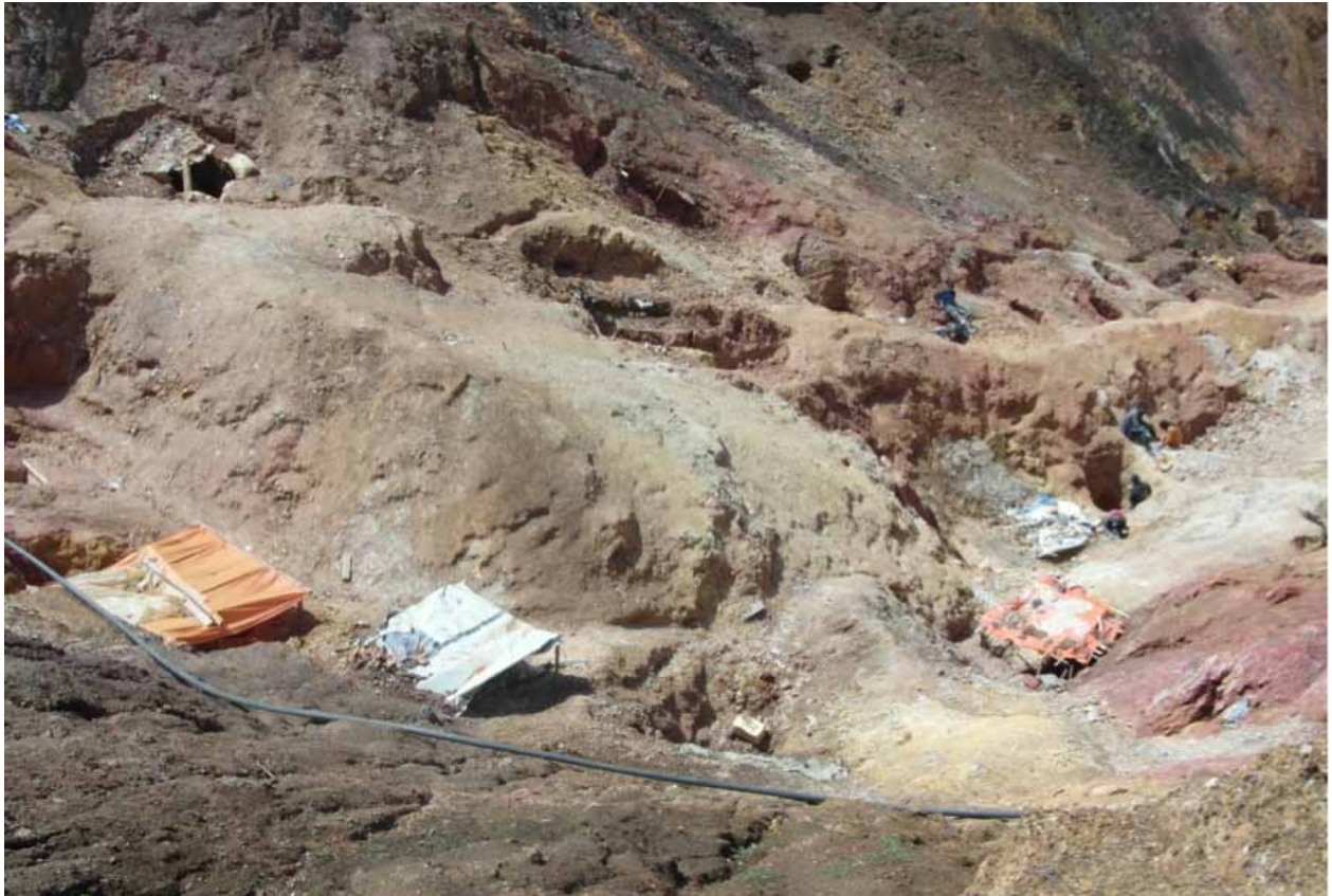
F: Tunnels on southwest side of the mine with pit shelters and water pump visible (IPIS, 2015)
