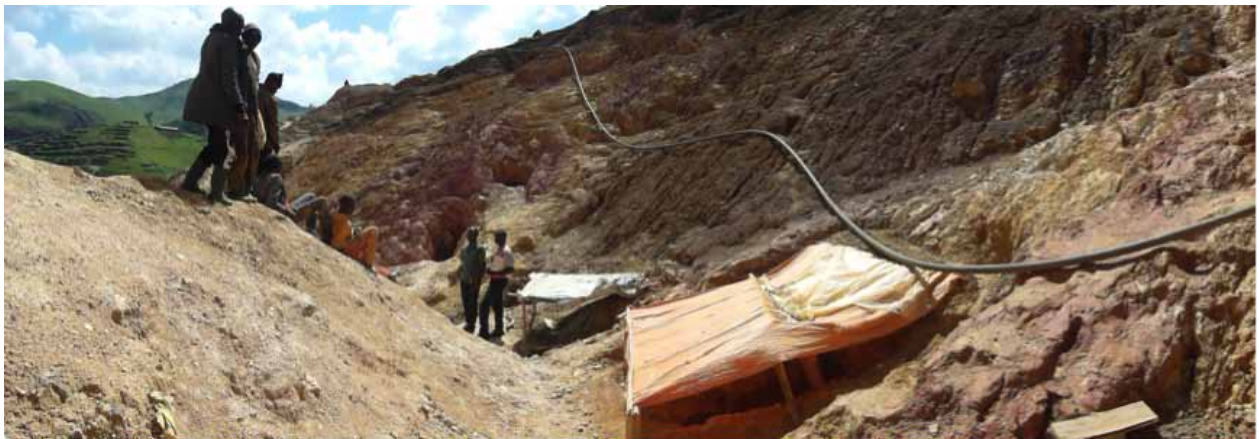
H: Shelters over mine shafts to prevent water ingress (IPIS, 2015)
