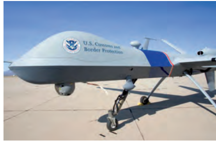
Predator Unmanned Aerial Vehicle (UAV) used for Border Control (Credits: US Customs and Border Protection).
