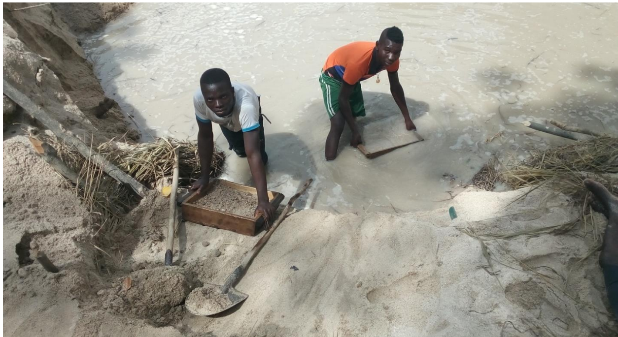
Photo 28: Gravel screening at the Kolongo diamond site.
